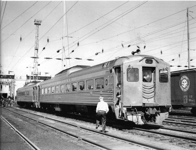
This fantrip couldn't have gotten much closer to the float bridge just east of RDC-2 3121 at Bay Ridge Yard in 1956. Freight trains were assembled here for New Haven electrics to move to New England after cars were floated from PRR Greenville Yard. LIRR BB3 units put trains together, but in later years ALCo diesels handled these chores, when the catenary in the yard was de-energized. It must be high tide; notice how high the float bridges have been raised. (Author's collection)
