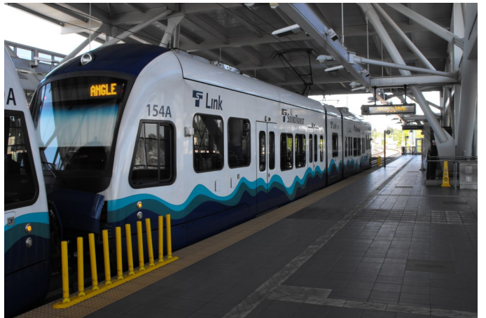
Sound Transit’s Kinkisharyo LRV fleet is being supplemented by 152 Siemens S70s, scheduled to be delivered starting in 2019 for further expansion. Central Link uses 1,500-volt d.c. vs. the 700/750 volts more commonly found to avoid the need for numerous substations.
