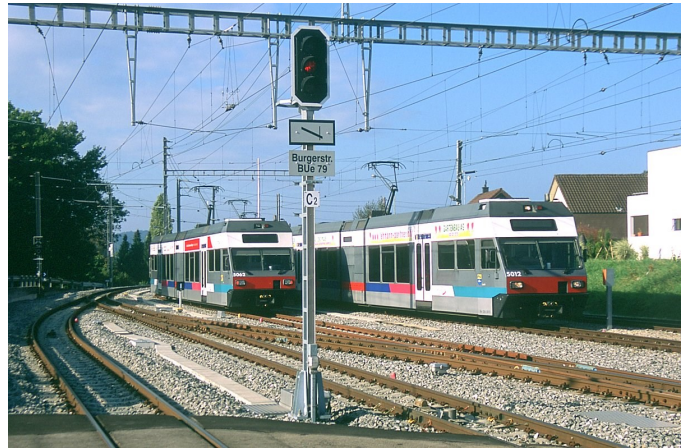
Two views of the BTI's modern 1997-built cars at Tauffelen. The left view shows a Biel-bound unit accelerating after pausing to drop and receive passengers. The right view shows the yard with two of the cars laying over before the afternoon rush hour. The BTI was the first recipient of these Stadler designed and built cars, which with their control equipment between two articulated sections, had become very popular in Switzerland. The diesel version was first placed in service on NJ Transit's River Line.
