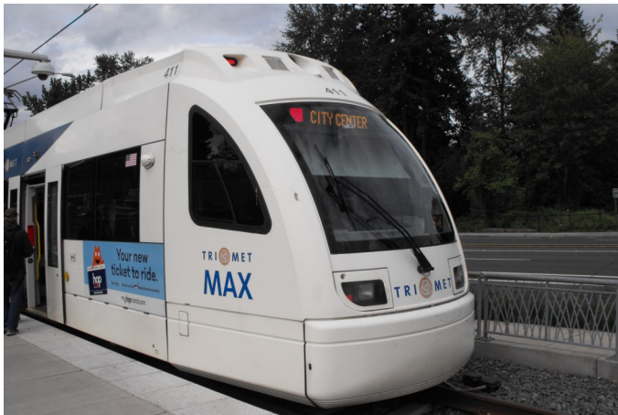
The front of TriMet MAX Light Rail Siemens S70 car 411. The S70s used by TriMet are single-ended and run in somewhat married pairs.
