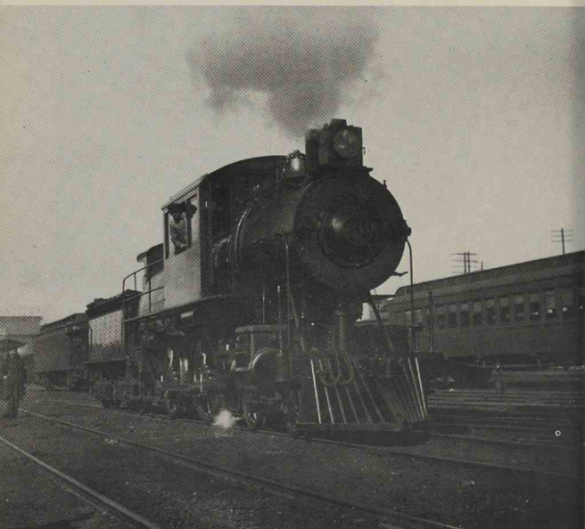
Engine #153, a 2-8-0 freight Camelback, built by Brooks in 1898. (Gene Collora) (Top) Engine #54 at Long Island City, a 4-4-0 Rogers engine of 1882 rebuilt to a Camelback. (ex.-122) (Ziel) (Bottom)
