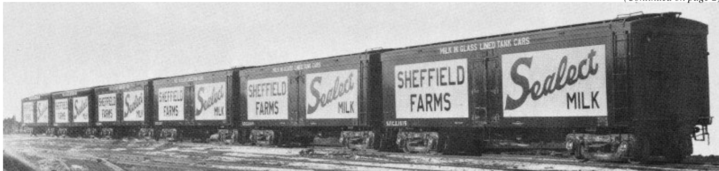
Bulk milk tank cars on the LIRR built by General American Pfaudler in 1928
