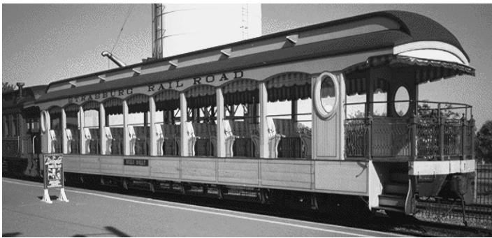
Bob Bird's modeling subject — Ex Boston & Maine coach 856 built by the Pullman Company in 1896 and rebuilt by the Strasburg Railroad as the Hello Dolly car for the movie.
