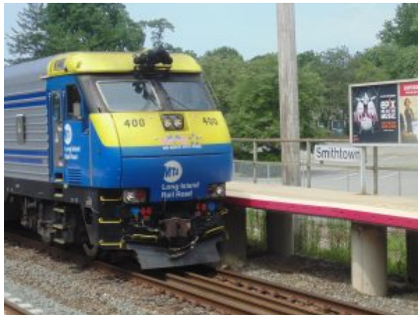
Figure 8. LIRR EMD DE30AC diesel locomotive at Smithtown Station (2013: Collection of Derek Stadler)
