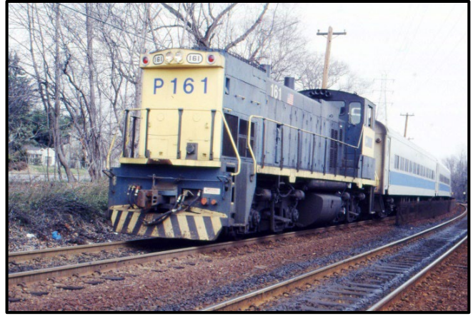
LIRR Electromotive Division MP15 number 161 converted for push-pull service, April 2, 1995, by E.M. Koehler.
